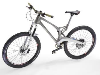
The Future - 3D printed bicycle by Renishaw and Empire Cycles
