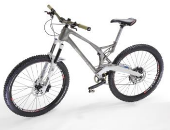
The Future - 3D printed bicycle by Renishaw and Empire Cycles
